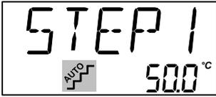
The calibrator will now work towards the given set-temperature. An audible alarm will be emitted once the calibrator is stable.
