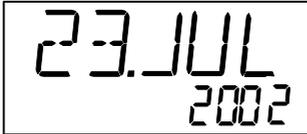
The calibration date will be displayed for approx. 2 seconds. The initialisation process has been completed and the calibrator is ready for use.
