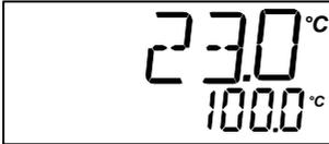
The starting point is the last chosen test-temperature (even if the instrument has been switched off).
