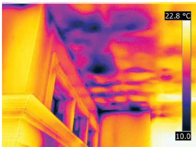
Quickly detect moisture intrusion and building deficiencies
