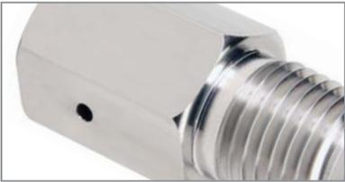
CPF Fittings and Hoses\* are machined in High-Strength 316 Stainless Steel to operate with a 4:1 Safety Factor at 10,000 PSI/700 bar/70 MPa. The Self-Venting Weep Hole alerts you, by leaking gas or test fluid, **BEFORE** you fully disconnect from a pressurized system. You'll never make *this mistake* again.
