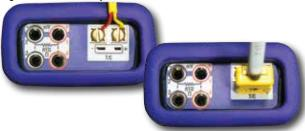
Simulating or reading RTDs uses copper wire.
