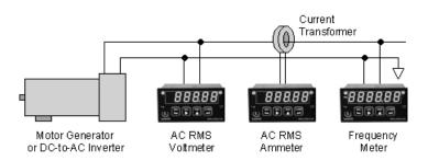
Using Laureate Meters and Counters to Instrument an AC Line
