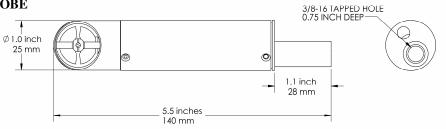
CABLE ATTACHED -5 FEET LONG (1.5 meters) TERMINATED WITH CONNECTOR FOR ATTACHING TO INSTRUMENT
