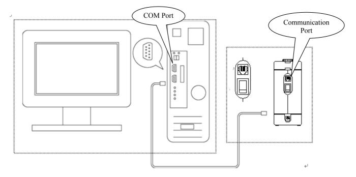
(2) If the computer is not equipped with a COM port, a USB-RS232C converter can be used to connect the instrument to the computer.
