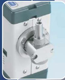
Impactors for 10 and 4 micron cut off
