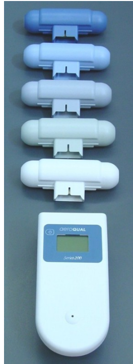
Sensors heads are interchangeable
