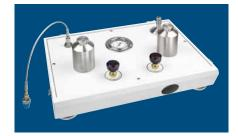
separation. Driven by a pneumatic pressure source (nitrogen bottle) and controlled by needle valves, high pressure gas is balanced against the liquid in a hydraulic deadweight tester through a series of fluid traps.
