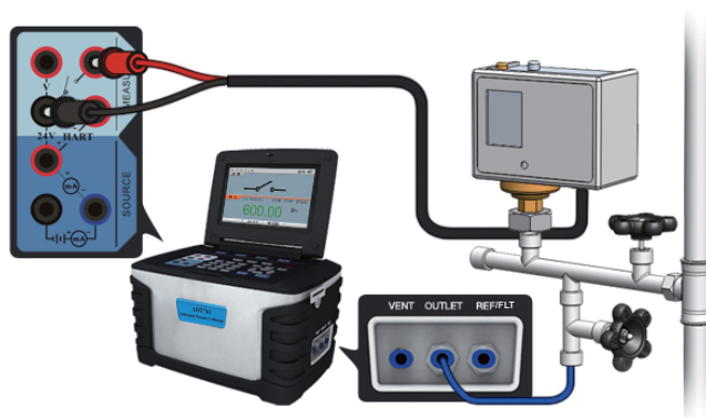
Figure 3-18 Calibrating a pressure switch
