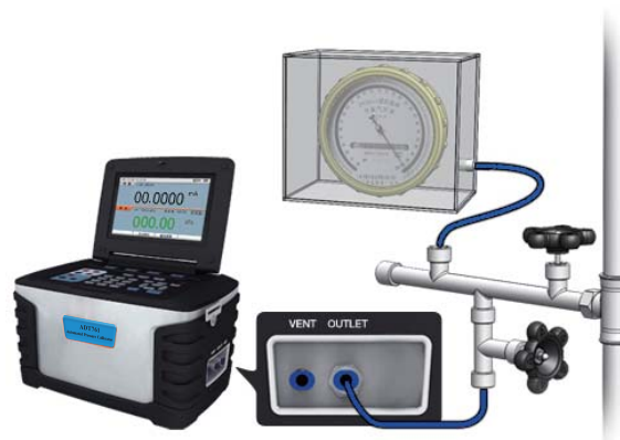
Figure 5-3 Calibrating an aneroid barometer
