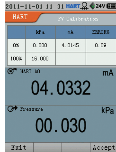
Figure 11 10 HART PV Calibration Process
