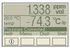
b. Display Mode - *Dual Dewpoint Units and Temperature* of gas under measurement. Note the status bar indicates that the measurements are pressure corrected, as requested these are computed what they would be at atmospheric pressure. The sample temperature is 20°C.
