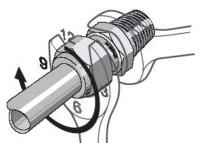
Rotate the nut finger-tight, then while holding the fitting body steady with a  $^9/_{16}$ " wrench, tighten the nut three-quarters turn with a  $^7/_{16}$ " wrench -
