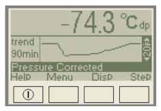
c. Display Mode - Single Dewpoint Units and Graph of the measured dewpoint in the last 90 minutes, with a span of 20°Fdp. This is also pressure corrected. The graph span will automatically resize to accommodate the minimum and maximum measurements in the last 90 minutes.
