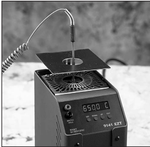
Figure 1 Heat shield installed on 9141 calibrator
