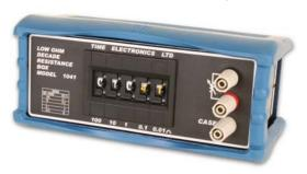
The **1041** is a compact, robust, and accurate decade resistance box designed for applications in both industry and education. With its low resistance ranges the 1041 is particularly suitable for simulation of platinum resistance thermometers.
