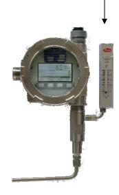
The PhyMetrix Sample System is designed to perform the measurement close to atmospheric pressure by regulating down the sample gas. This decreases the likelihood of liquid contaminants (they are vaporized) as well as it reduces the concentration of water vapor and of  $H_2S$  thus the likelihood of corrosives forming is also reduced and sensor life is prolonged.
