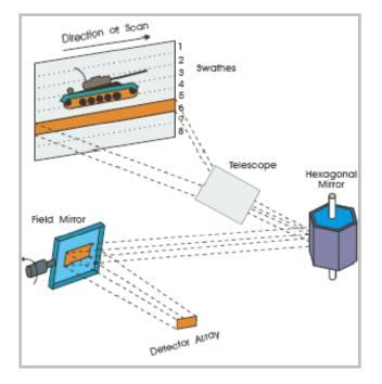
2nd generation thermal imagers contained twodimensional arrays with several columns of elements (12 x 12). These thermal imagers still required scanning in one direction and complex electronics to improve the signal-to-noise ratio.
