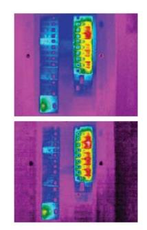
Comparison of two images, one taken with a 320x240 camera (top) and the other with a 160x120 camera (bottom) – Snell Infrared
