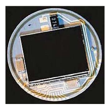
320x240 pixels detector array mounted onto a carrier substrate. The total size of the chip is  $11 \times 14 \text{ mm}$ .
