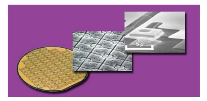
Microbolometer detectors can be operated at room temperature and therefore do not require cooling.
